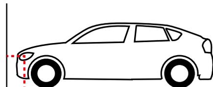
3. Connect the center points between headlights in a straight line, using chalk or tape. This will create your X axis line. **NOTE: Use a straight edge and a level to make sure this line is straight.**
