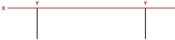
5. Reverse your vehicle in a straight line so that the front of the headlights are 7.62 meters (25 feet) back from the wall.
