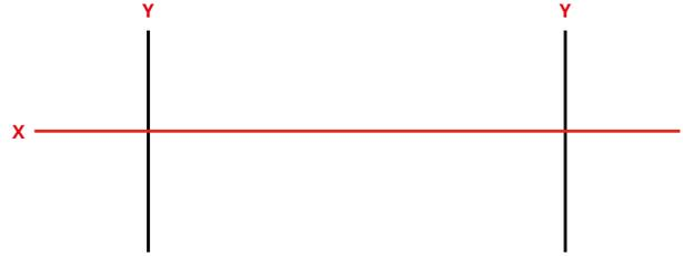
The goal of this sheet is to aim BOTH of your headlights so that the center of the **Hot Spot** is at the v of the horizontal X and vertical Y lines you have drawn. The following directions illustrate the process and proper aiming of headlights.
