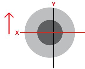
8. On the same headlight, adjust the same headlight horizontally until the alignment point is even with the Y axis.
