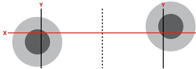
7. Using the alignment mechanisms in your vehicle, adjust one headlight vertically until the alignment point is even with the X axis.
